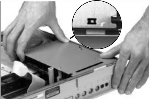
Inserting the PowerPro/Adapter combination in the PDS connector.
