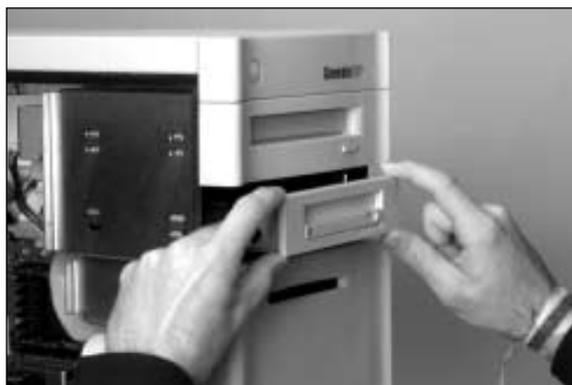
*Inserting 5.25" Device*
