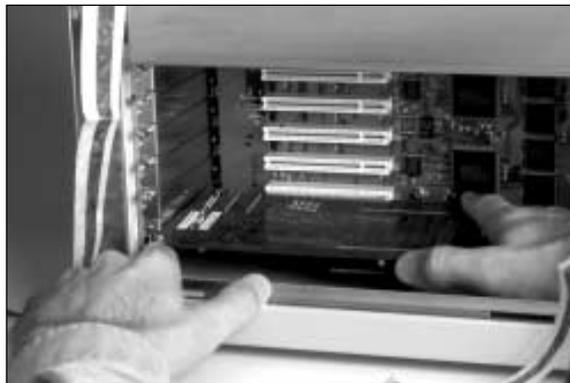
*Installing PCI Card*
